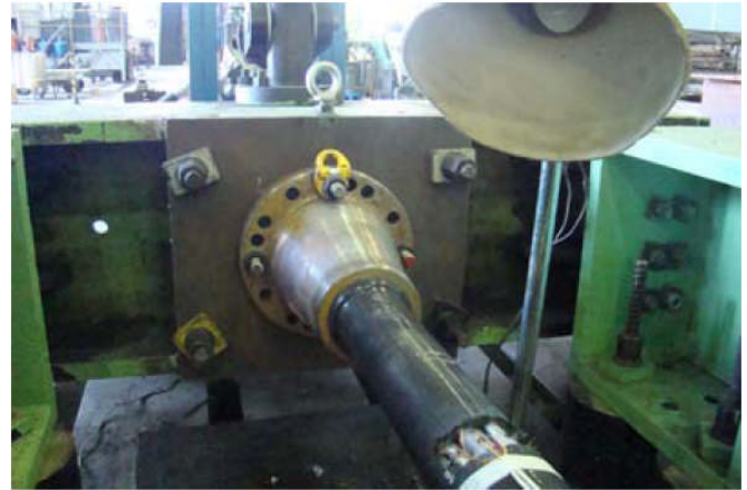
Figure 3 – Partial view of the test bench showing the umbilical sample and one of the armour pots connected to the fixed end-plate.
