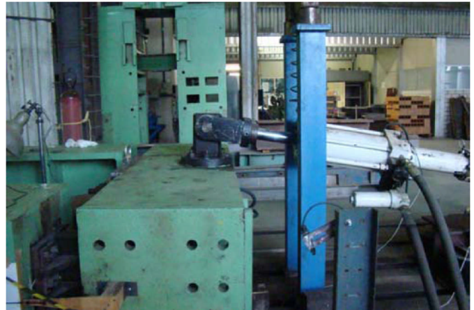
Figure 4 – Partial view of the test bench showing the hydraulic actuators at the active end-plate.
